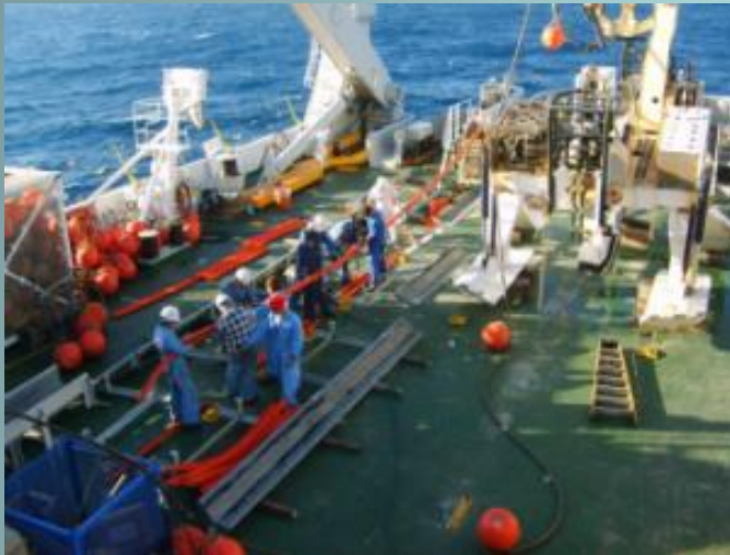
Urduct installation aboard the CS Tyco Reliance that took place 7 th February
